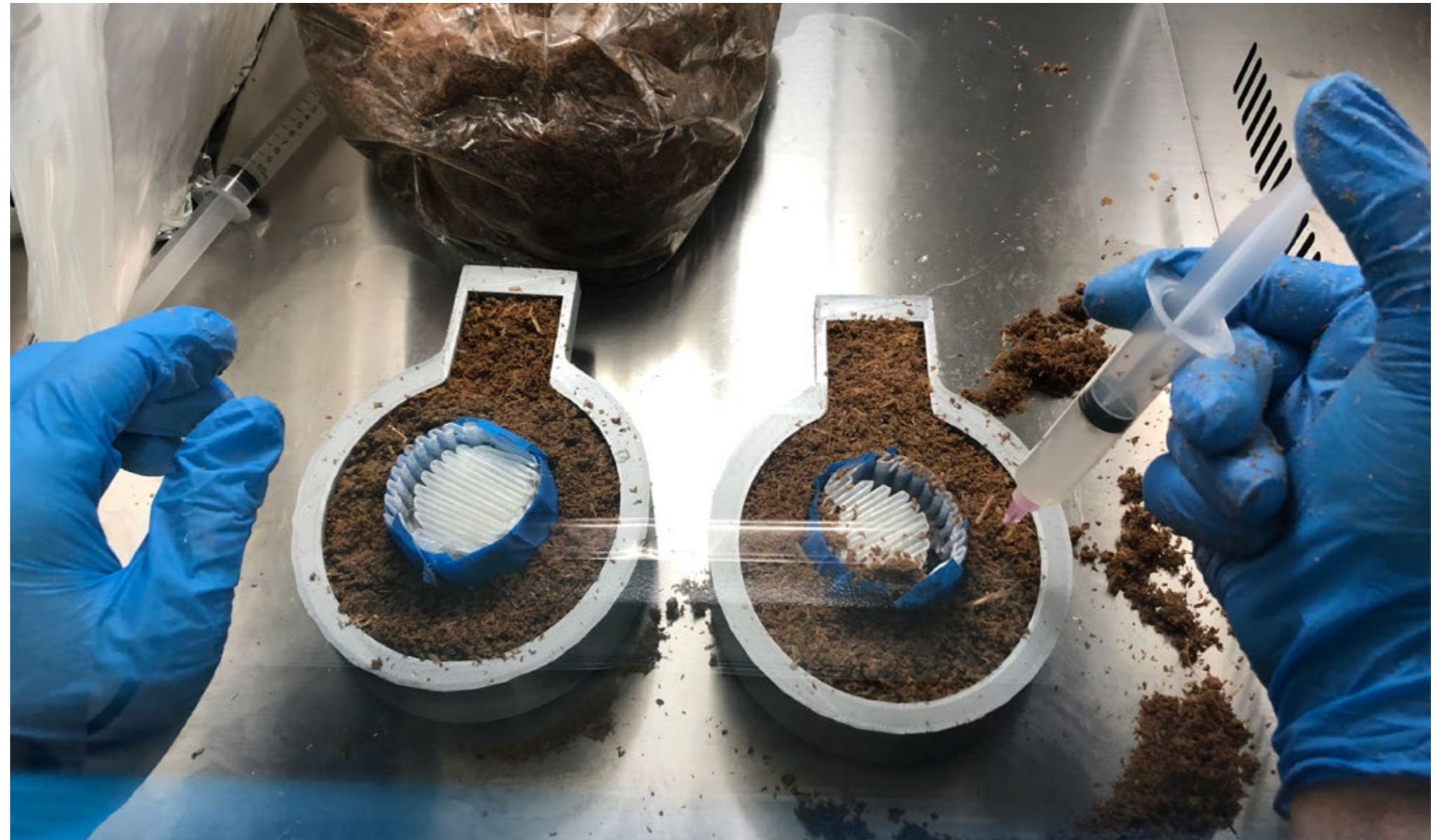
Filling forms with substrate while inoculating the substrate with a mycelium culture
