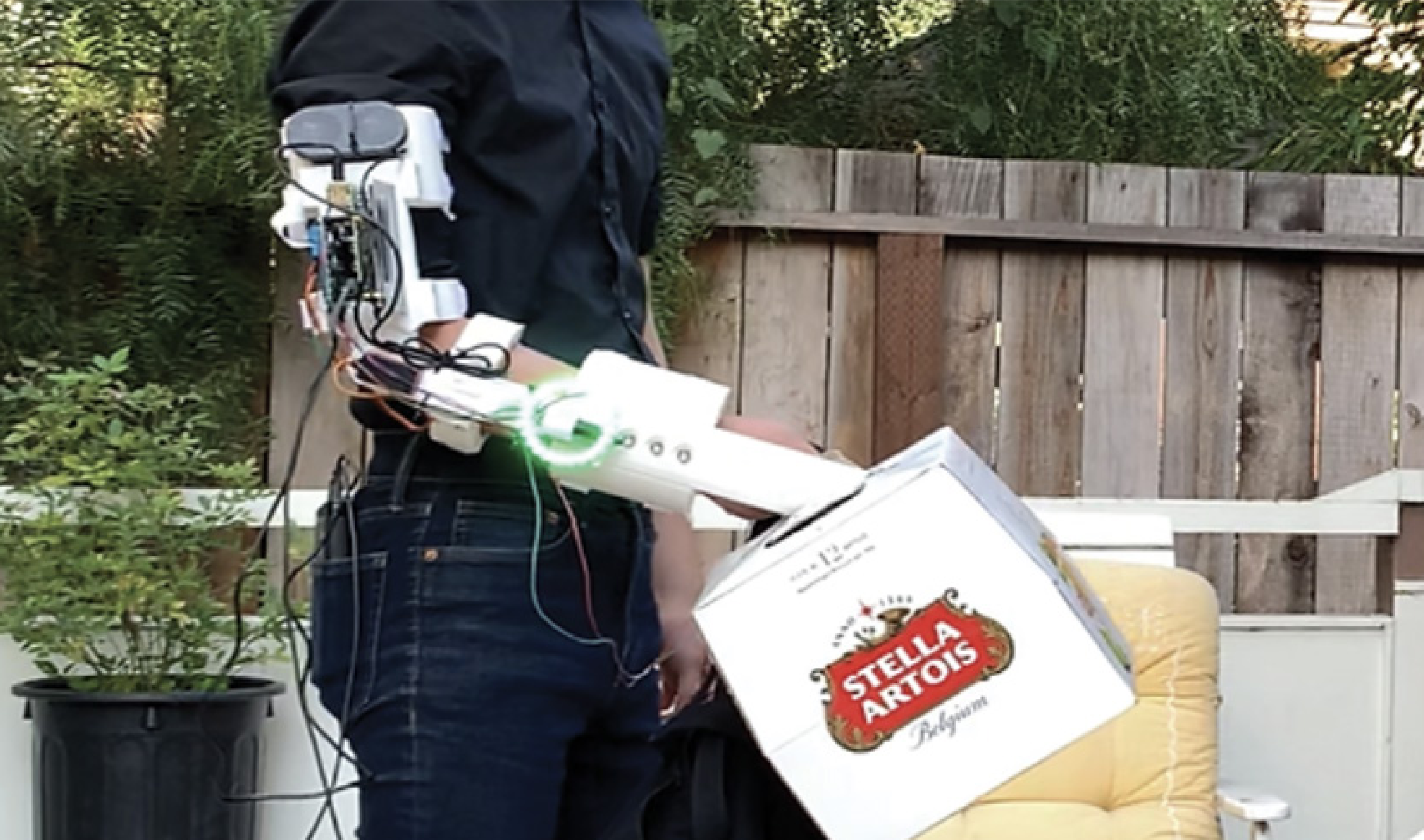
1st Prototype Equipped with a raspberry pi to mainly explore all different functions the arm can perform. Limited lifting capacity.
