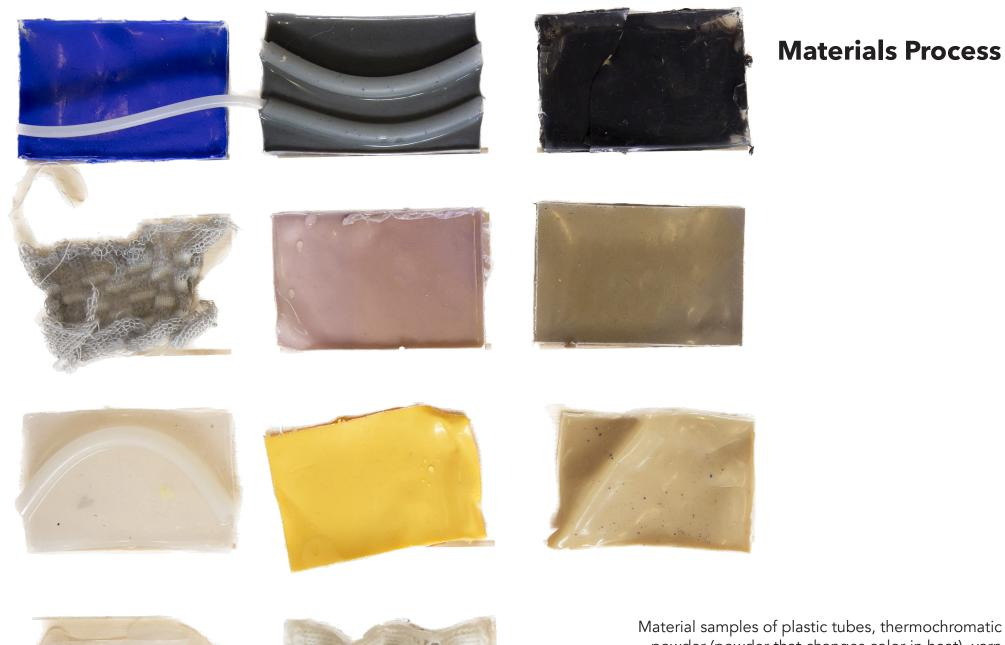
Material samples of plastic tubes, thermochromatic powder (powder that changes color in heat), yarn and conductive thread embedded into silicone. The experiments were to help better undersand what components to include in the outer skin of the silicone placenta.
