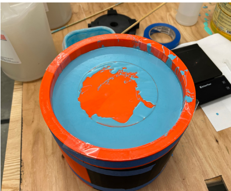
Platinum cured silicone rubber mixed and poured into the 3D printed casting mould. Figure 06.3
