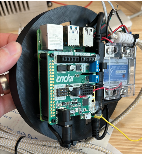
Raspberry Pi, Cricket Hat for Capacitive Sensing and a solid state relay installed on a 3D printed electronics mount.
