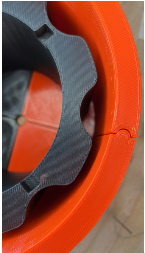
A section of the 3D printed Fungal-Form cooler placed within a 3D printed casting mould. Figure 06.2
