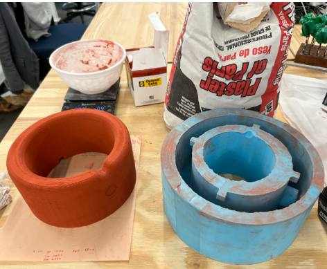
Terracotta segment removed from a silicone mould.
