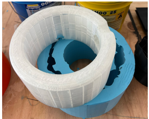
A section of the 3D printed Fungal-Form Cooler removed from a Platinum cured silicone mould. Figure 06.4
