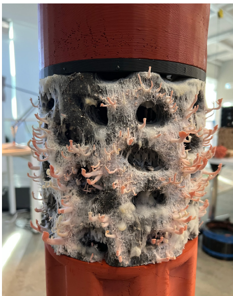
Photos showing FungalForm loaded with a Pink Oyster MycoCore.
