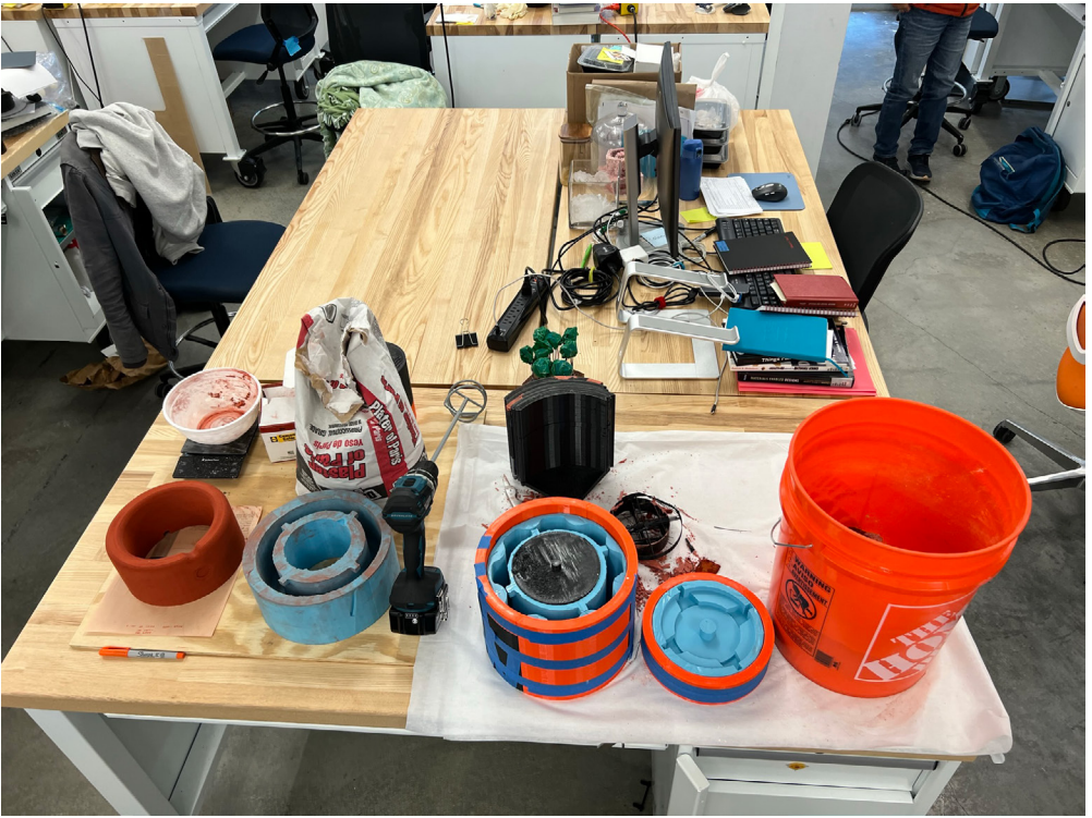
Terracotta (Plaster of Paris and red/black concrete pigment) casting set-up.
