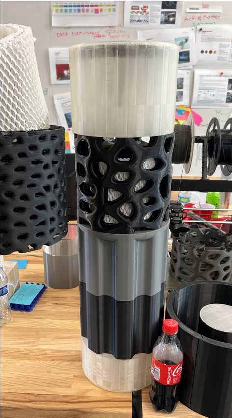
Final 3D printed scale 1:1 FungalForm Cooler Figure 06.1
