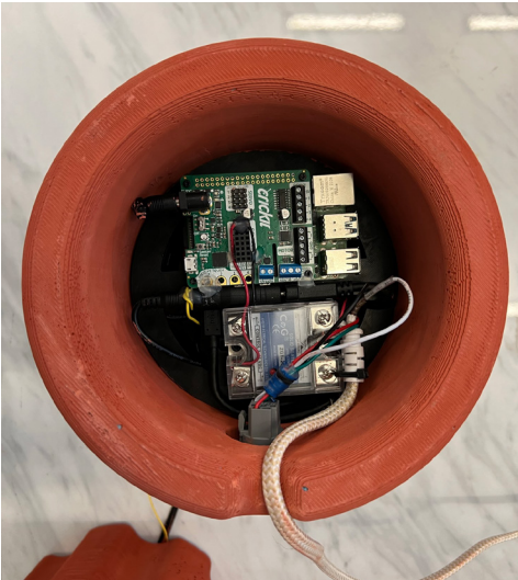
Electronics mount with electronics attached installed in the base segment of FungalForm.
