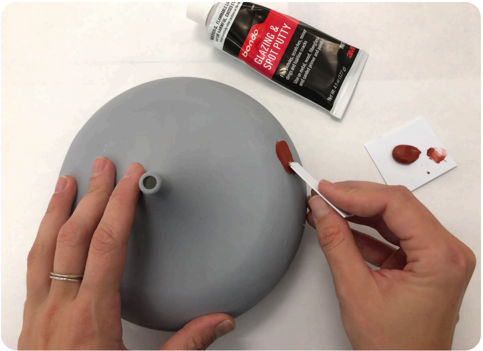
Applying glazing putty to final 3D-printed and primed models.
