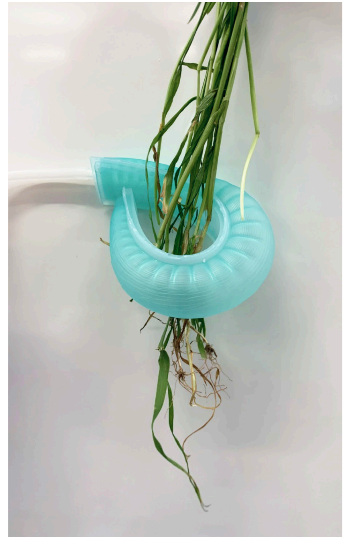
▲ Testing with air-pump and soft robot made with dragon skin.
