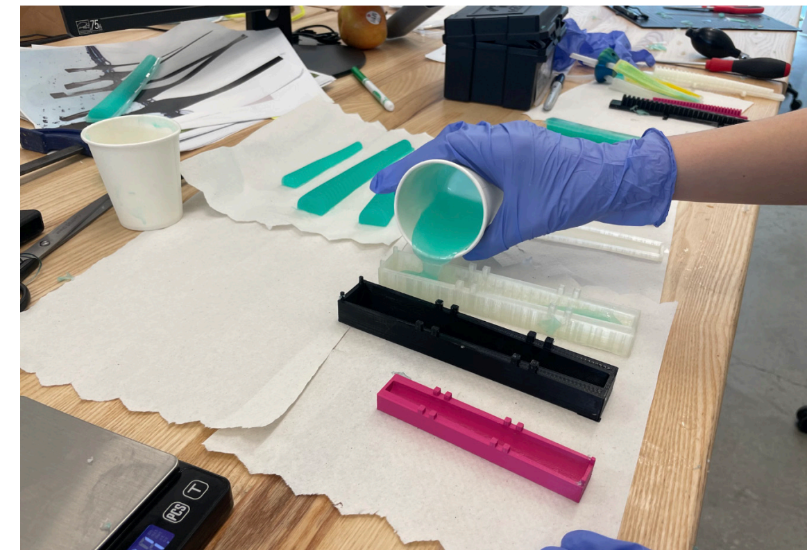
▲ Printing out with 3d model to make molds and pouring silicions
