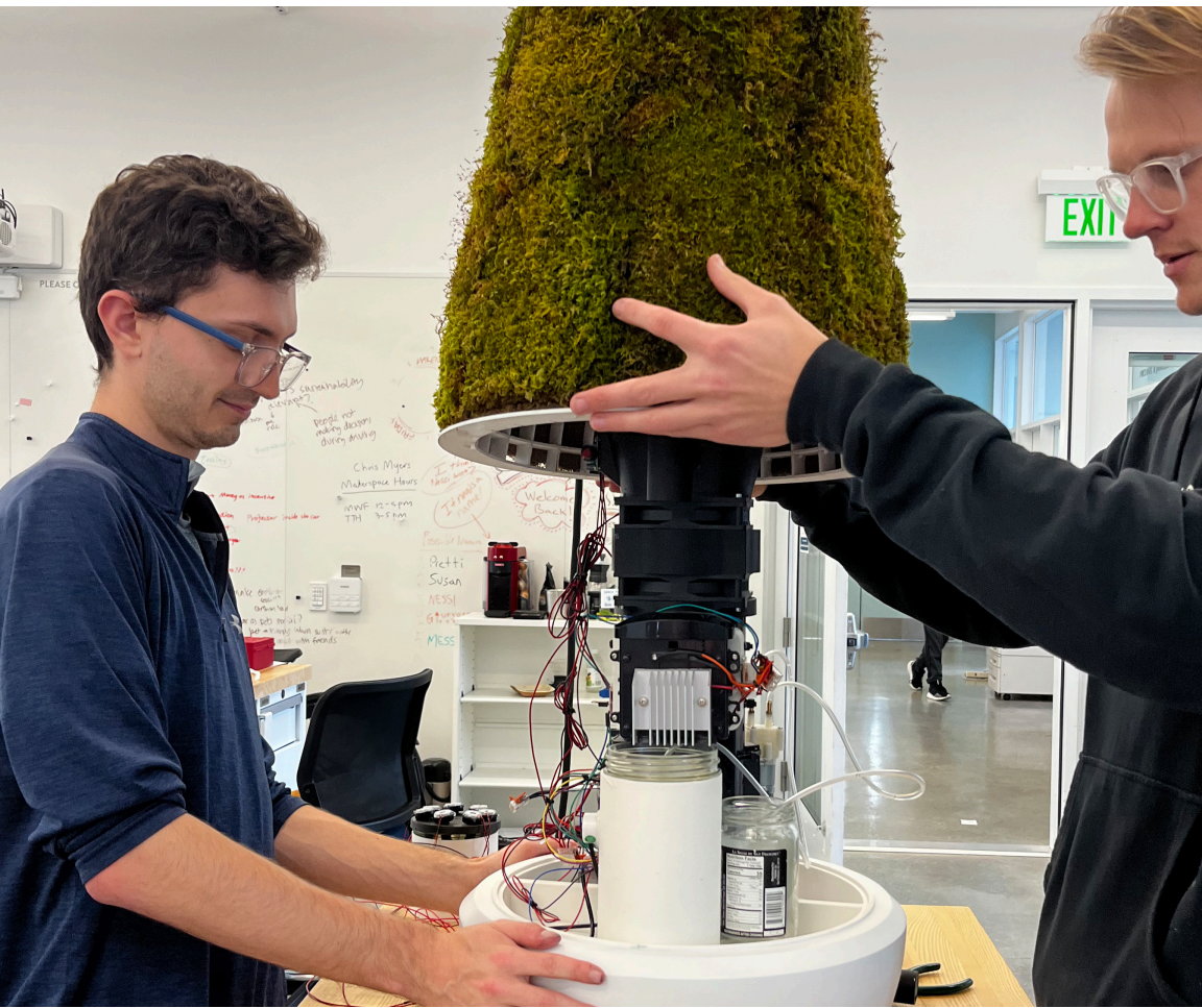
Placing the moss purification layer
