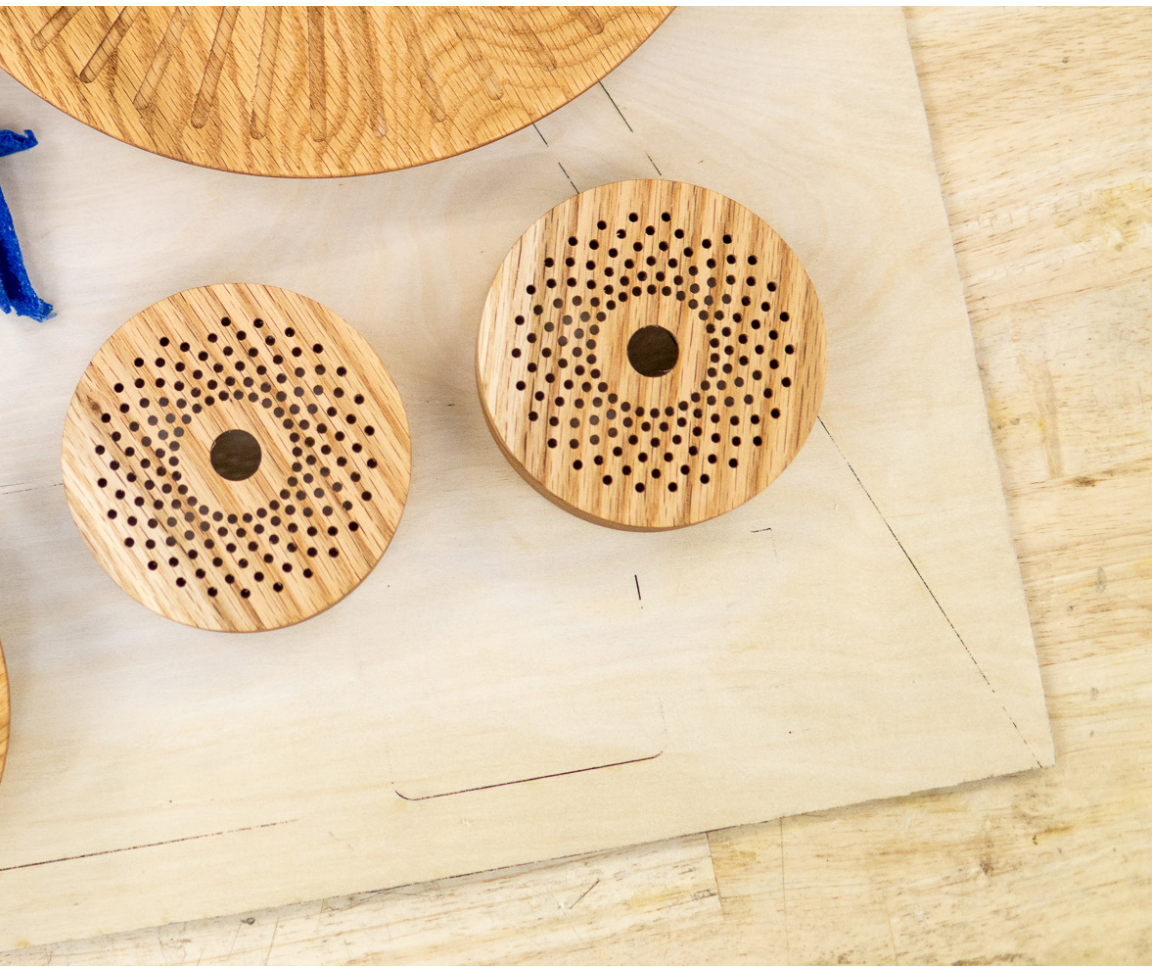
Housing for air quality monitors
