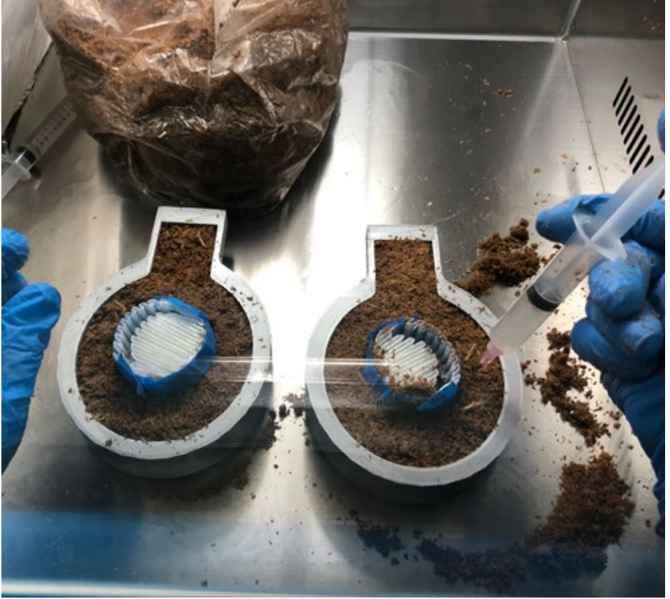
Innoculating the first prototype molds with reishi mycelium culture in Dedrick Siddalls laboratory, March 2022
