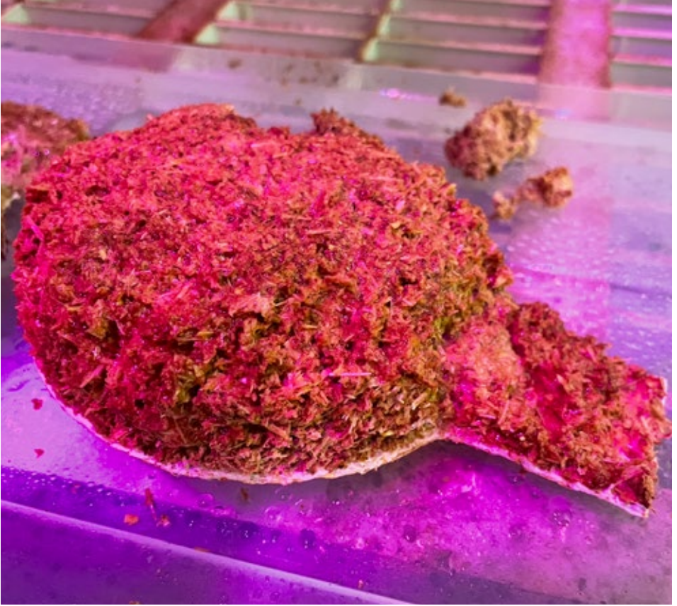
Failed first prototype as the substrate did not receive enough oxygen due to wall thickness of the mold, May 2022
