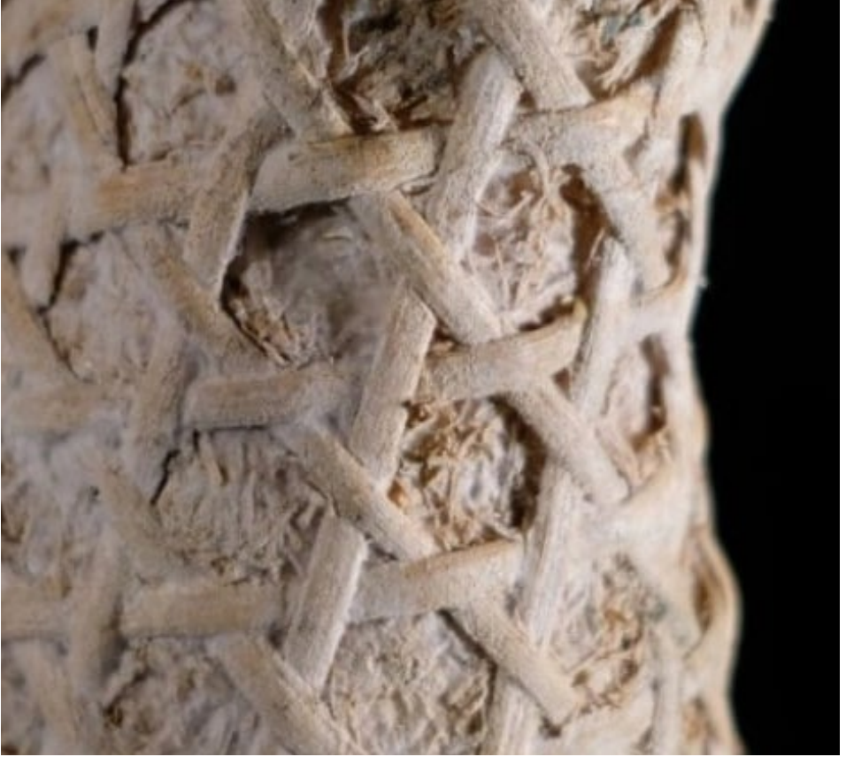
Mycelium as potential future building material in architecture, Royal Danish Academy, Phil Ayres
